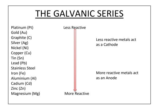
Generally, the closer one metal is to another in the series, the more compatible they will be, i.e., the galvanic effects will be minimal. Conversely, the farther one metal is from another, the greater the corrosion will be.
